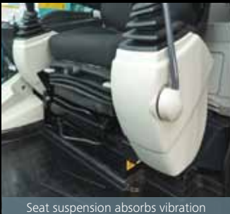
Seat suspension absorbs vibration
