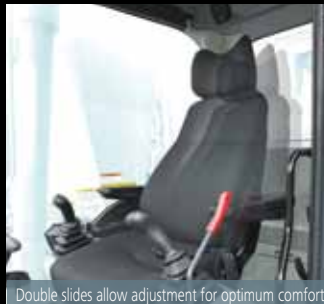
Double slides allow adjustment for optimum comfort
