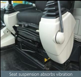
Seat suspension absorbs vibration
