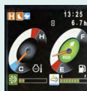
PM accumulation/ Urea accumulation display
