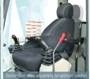
Double slides allow adjustment for optimum comfort
