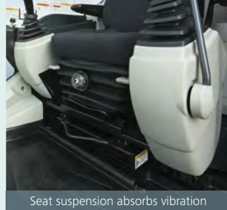
Seat suspension absorbs vibration
