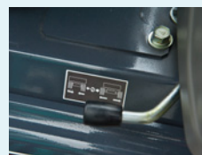
Crawler retract/extension lever
