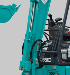
Boom cylinder rod guard
