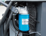
Cartridge type return filter
