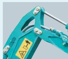
Bucket cylinder hose is housed inside the arm.
