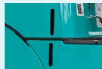
Fuel tank gauge
